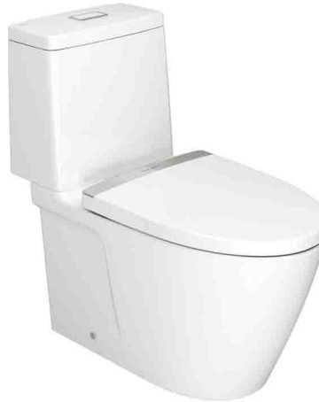
American Standard, Acacia Evolution Series TF-2307, Close coupled WC with soft close standard seat cover L740 x W376 x H760 mm (P-S Trap Connector -3" to 12"), Finish: Ceramic White (WELS Certified 3 Ticks) ** Suitable for HDB supply
